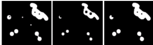
Fig 2 Opening: remove capex, isthmus and islands smaller than the structuring element
